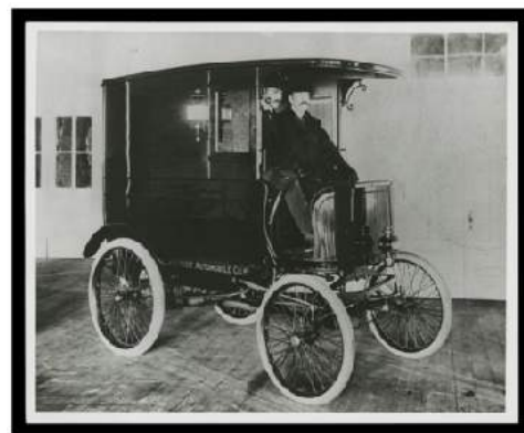
The company's first product was a gasoline-powered delivery truck engineered by Ford and completed in January 1900
